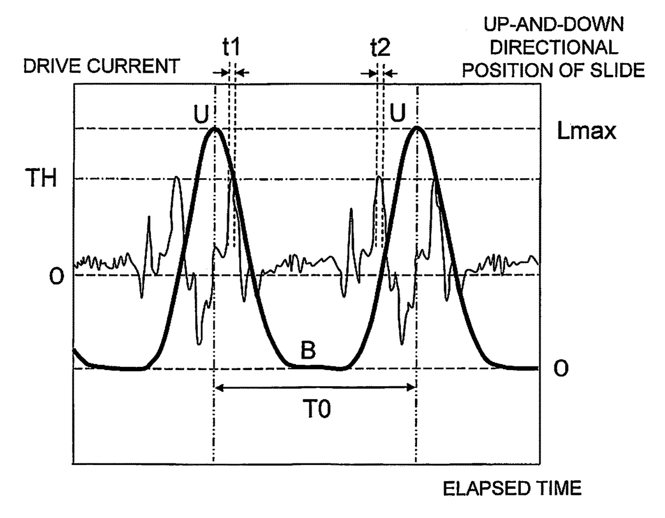
FINE LINE: DRIVE CURRENT BOLD LINE: UP-AND-DOWN DIRECTIONAL POSITION OF SLIDE
