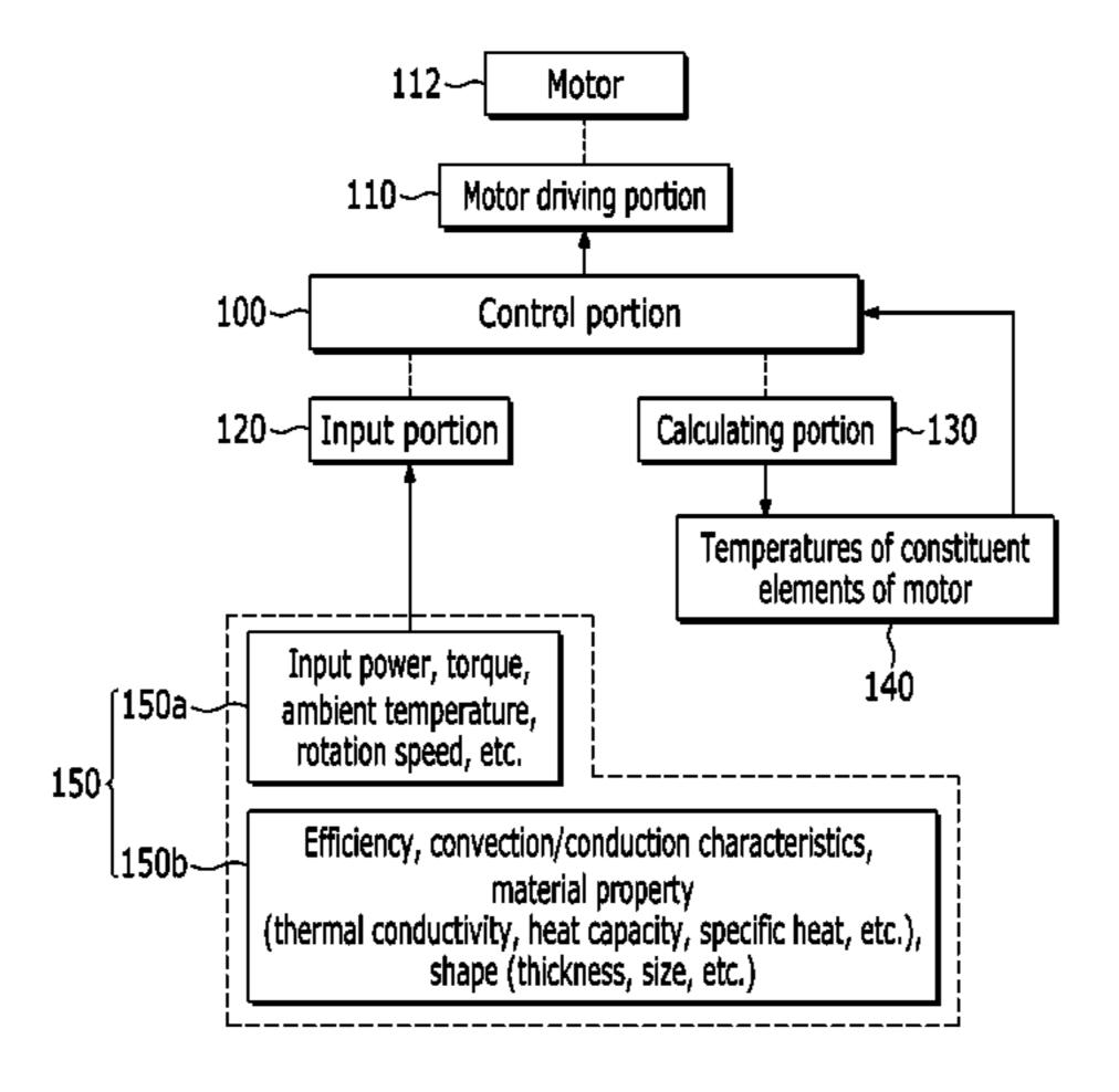
the input portion and convection or conduction characteristics between constituent elements of the motor, and calculating a temperature of each constituent element using the thermal equivalent circuit.
