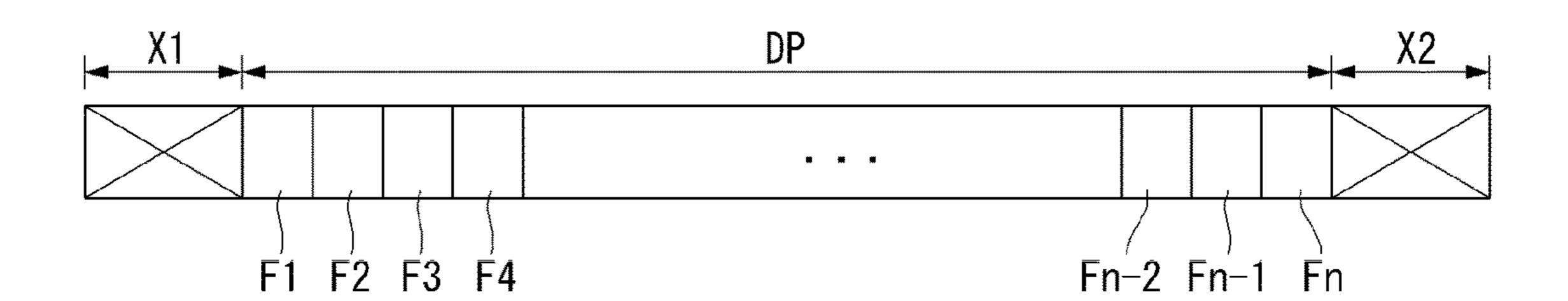
X1 or/and X2 : Vth EXTERNAL COMPENSATION OF THRESHOLD VOLTAGE
