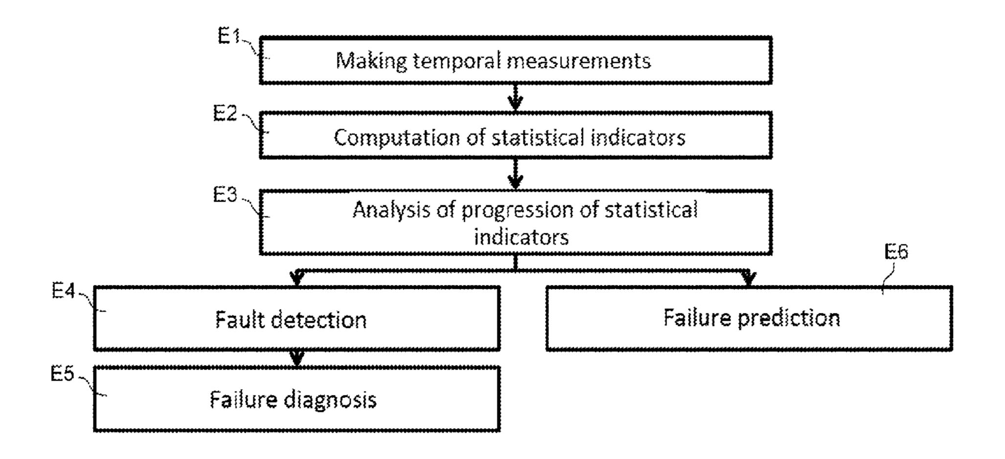
putation of one or a plurality of statistical indicators of the parameter measured and an analysis of the temporal progression of the statistical indicator(s) computed. The invention also applies to a computer program for the implementation of this method.
