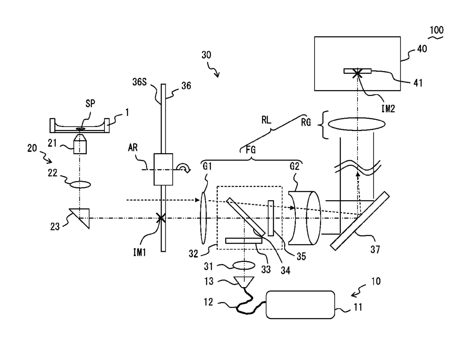
power and a rear group having a positive power, in this order from the rotating disk side, and is configured so that a luminous flux between the front group and the rear group becomes an afocal luminous flux. The disk scanning apparatus further includes a structure configured to make the distance between the front group and the rear group variable.
