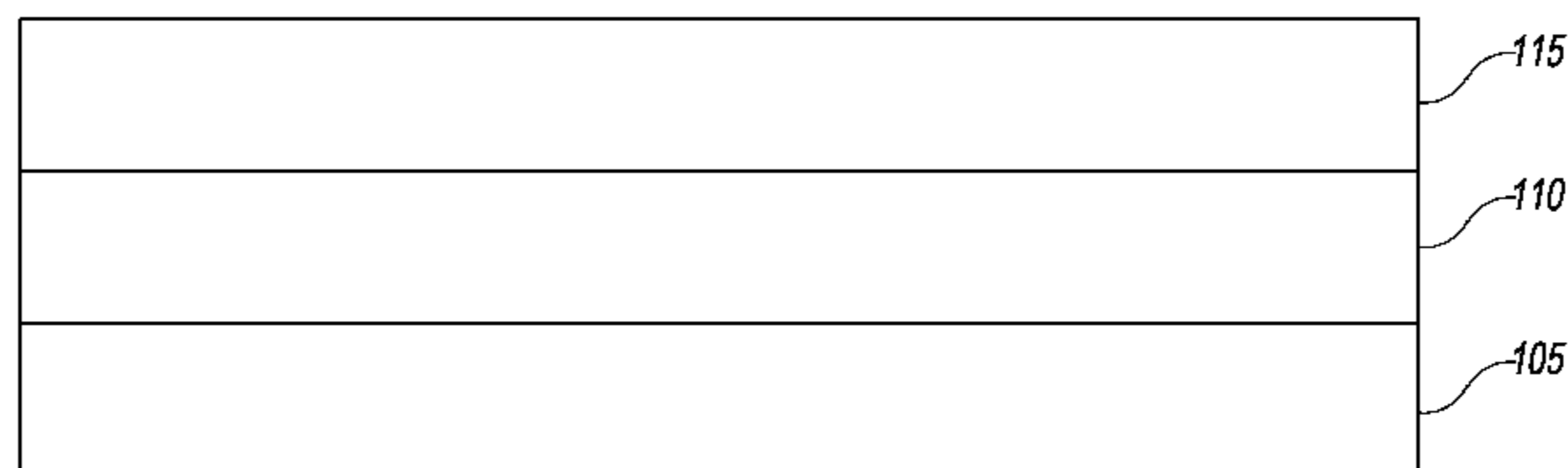
100 - Graphene Composite 105 - Substrate 110 - Photoswitchable layer 115 - Graphene Layer
