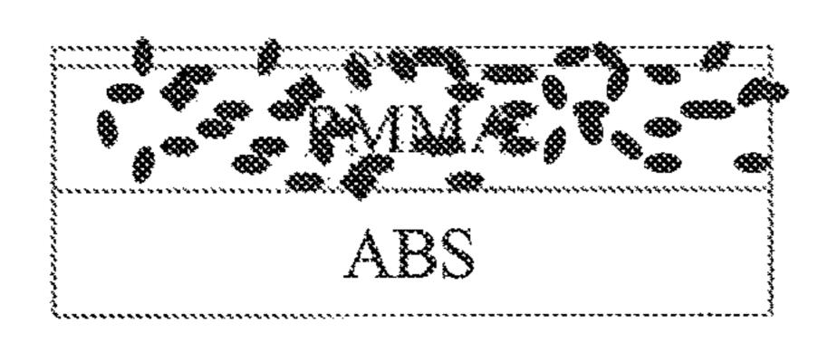
Produced by conventional coextrusion.
