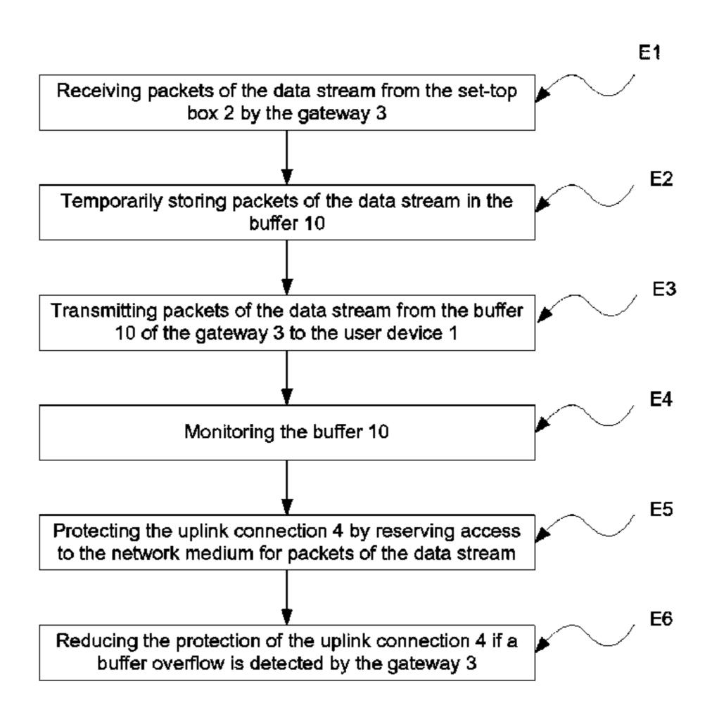
packets of the data stream of the uplink connection. Finally the network gateway comprises a control module that is configured to monitor the buffer and to send an instruction to the protection module to reduce the protection of the uplink connection if a buffer overflow is detected.
