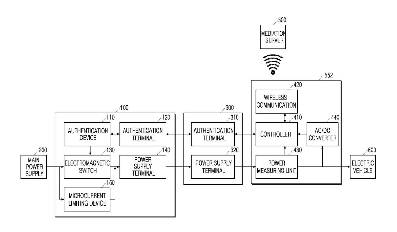
micro-current to flow when a power consuming device is connected to the user authenticating electrical outlet or connector. The authenticating power is obtained from the micro-current and is supplied from the outside via the authenticating terminal. When the electrical outlet operating password corresponds to the electrical outlet ID information, main power for the power consuming device is supplied from the main power supply to the outside.
