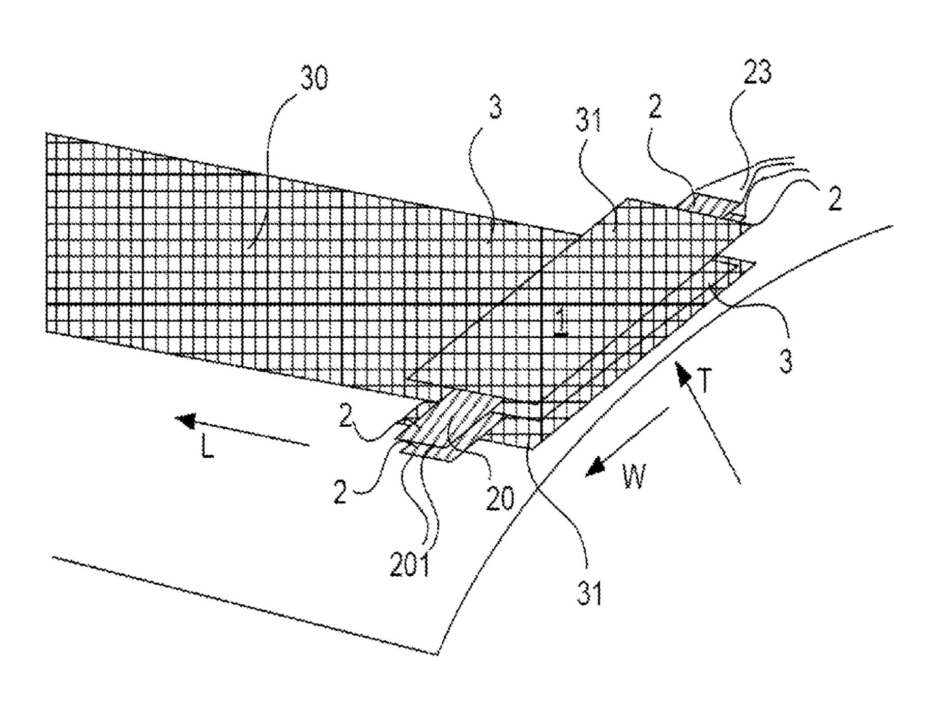
the strands substantially lie in one plane, adjacent to each other, and the ends of the strands extend, in the width direction (W) of the heating element, beyond the heating element, wherein the portions of the ends of the strands extending beyond the heating element overlap each other, and an electric joint is formed between the lateral faces of these overlapping strands.
