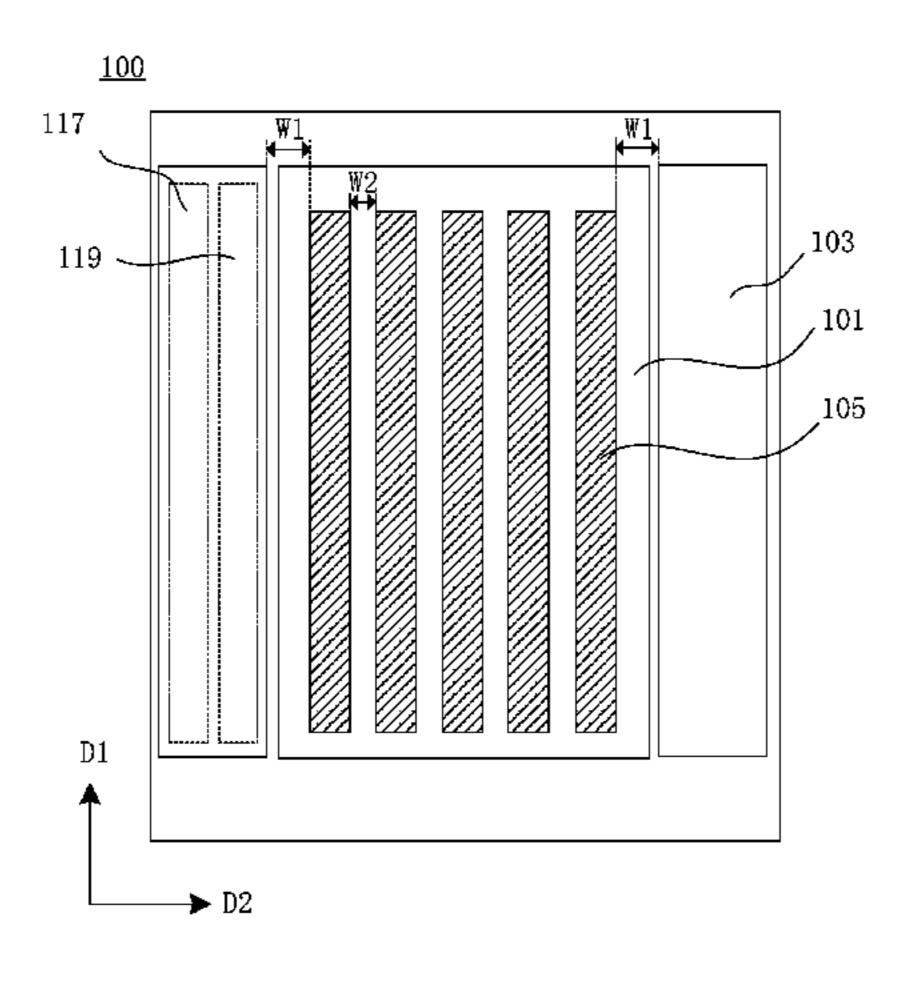
shaped touch control electrodes as a second width, the first width is greater than the second width.
