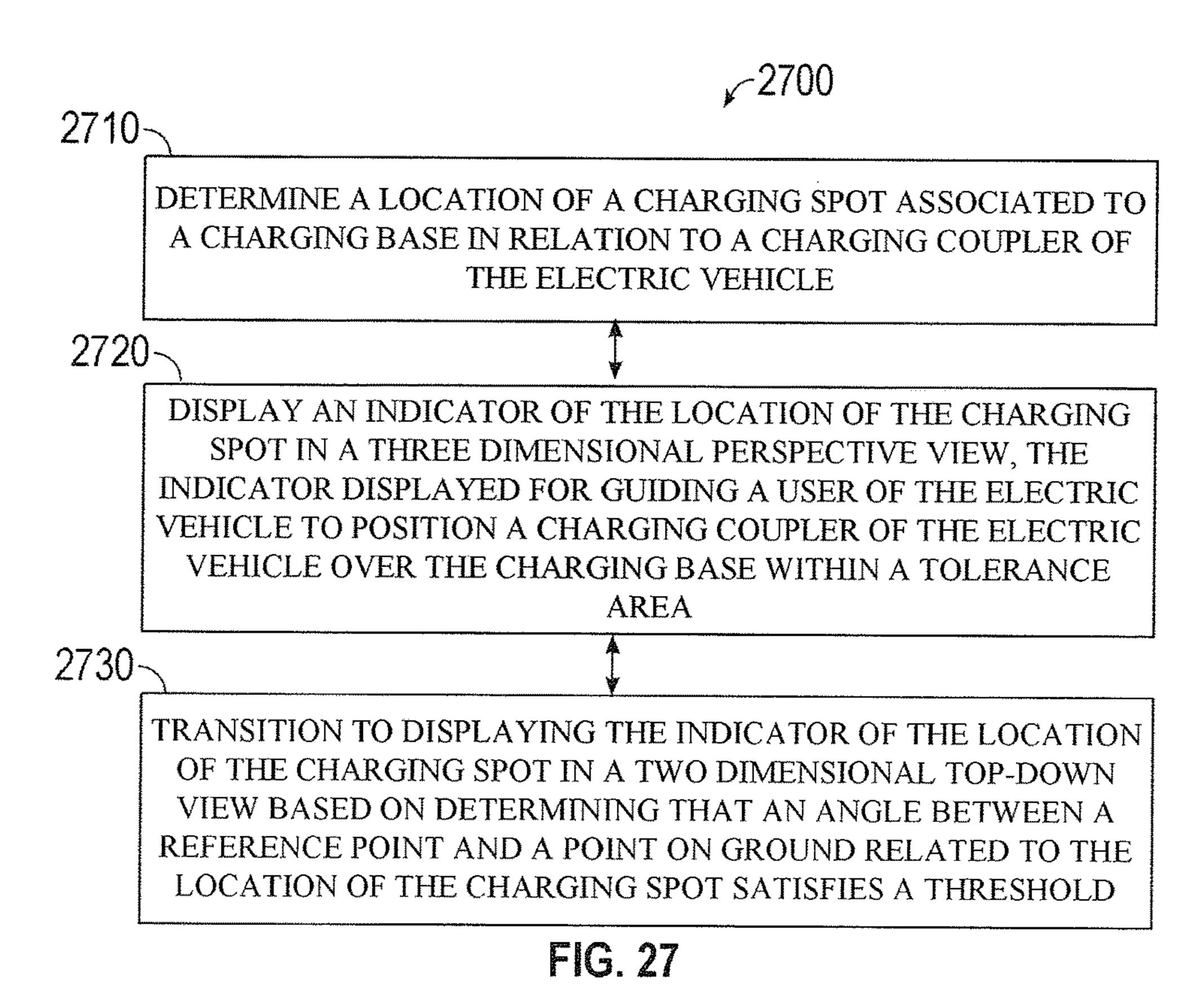
MEANS FOR DETERMINING A LOCATION OF A CHARGING SPOT ASSOCIATED TO A CHARGING BASE IN RELATION TO A CHARGING COUPLER OF THE ELECTRIC VEHICLE
