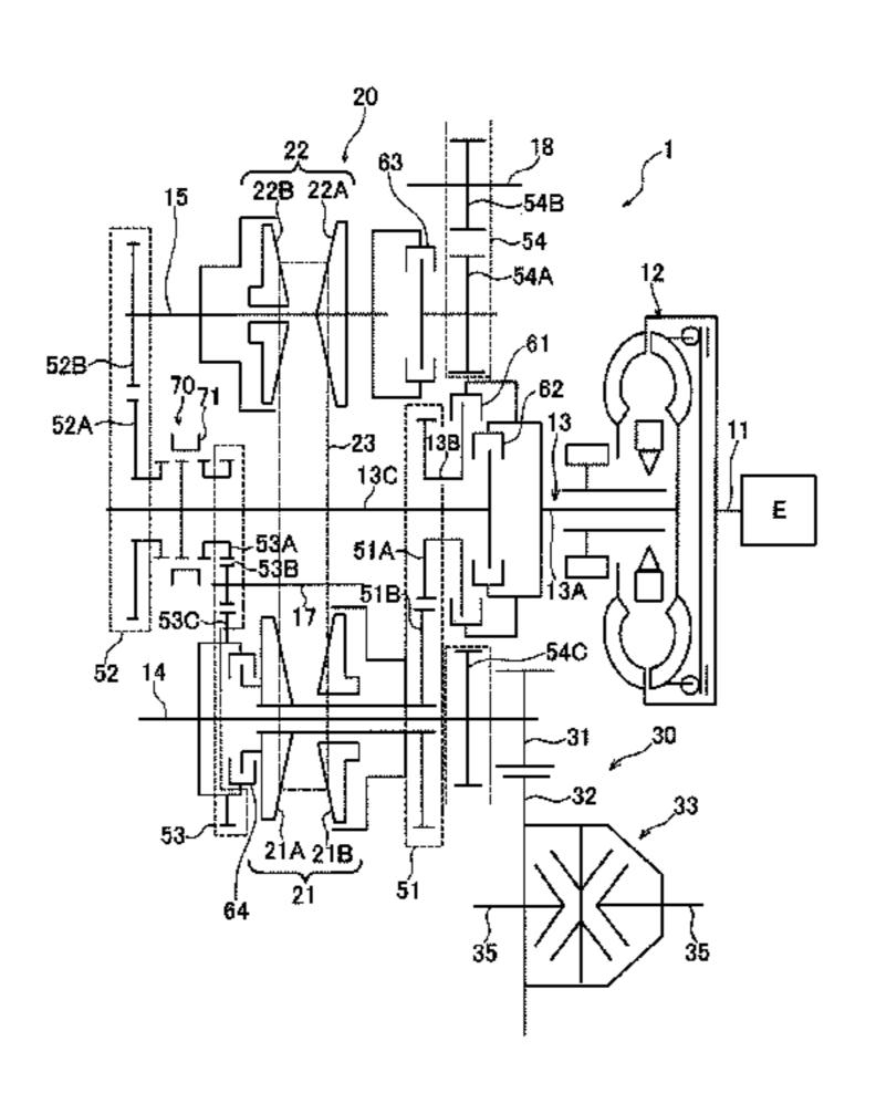
second output shaft. A fourth friction clutch is coaxial with the first output shaft.
