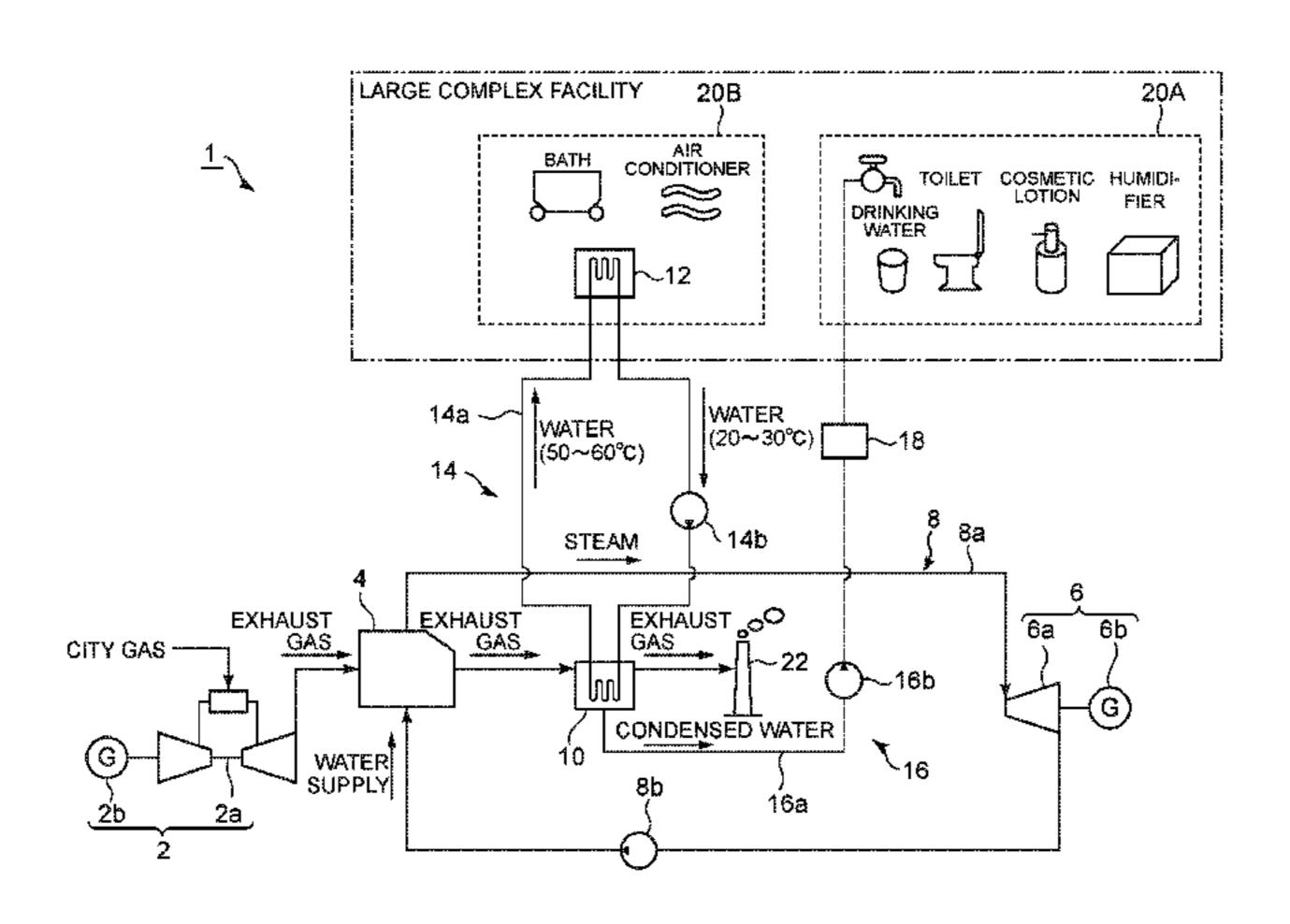
device configured to supply the heat medium heated by the condensation economizer to a thermal-energy recovery unit, and to return the heat medium to the condensation economizer after the thermal-energy recovery unit recovers energy of the heat medium.
