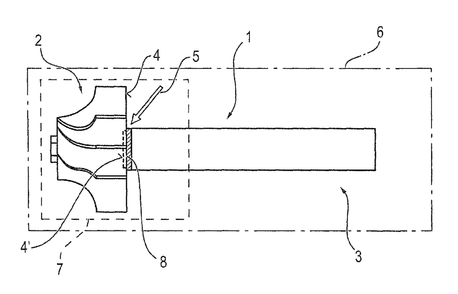
the shaft (3) by electron beam soldering by means of an electron beam (5).
