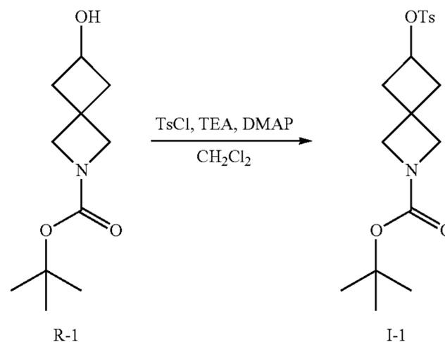
A solution of R-1 (5.0 g, 23 mmol) in CH<sub>2</sub>Cl<sub>2</sub> is treated with TEA (6.5 mL, 47 mmol) and DMAP (0.57 g, 4.7 mmol). The mixture is stirred for 24 h then concentrated in vacuo. The residue is dissolved in EtOAc and washed with saturated aqueous ammonium chloride and brine. The organics are collected and volatiles are removed in vacuo. The crude residue is triturated with Et<sub>2</sub>O and solid filtered and collected to afford I-1 (5.6 g, 65%) m/z 367.9 [M+].
