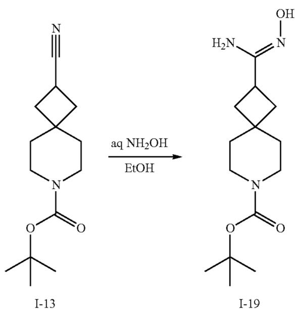
A solution of I-13 (422 mg, 1.69 mmol) in EtOH (8.4 mL) is treated with 50% (w/w) aqueous hydroxylamine (1.1 mL, 16.9 mmol). The solution is heated at 70° C. for 2 h then volatiles are removed in vacuo to afford I-19 (478 mg, quant) m/z 284.1 [M+H].
