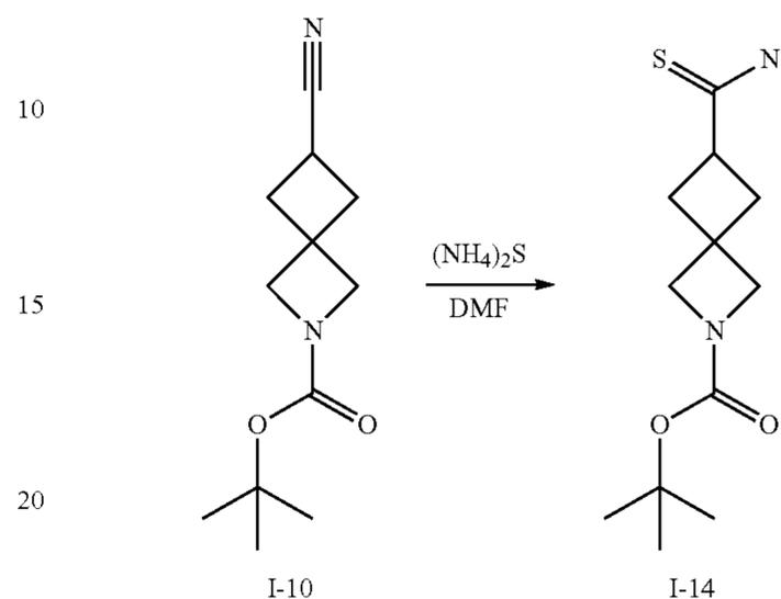
To a solution of I-10 (250 mg, 1.1 mmol) in DMF (2 mL) is added 20% (w/w) aqueous (NH<sub>4</sub>)<sub>2</sub>S (2 mL, 5.9 mmol). The mixture is stirred at ambient temperature for 17 h then diluted with water. The resulting white solid is filtered and collected to give I-14 (160 mg, 55%). m/z 257.0 [M+H]
