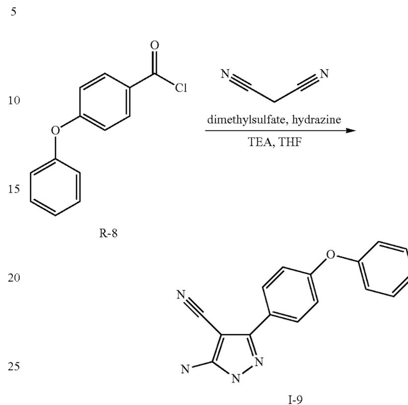
To malonitrile (7.55 g, 114 mmol) in THF (200 mL) at 0° C. is added sodium hydride (60% dispersion in mineral oil, 4.57 g, 114 mmol) slowly under a stream of nitrogen. After 10 min R-8 (27 g, 115 mmol) is added and the ice bath removed. The mixture is stirred at ambient temperature for 1.5 h then dimethylsulfate is added then heated at reflux for 2 h. The mixture is cooled to ambient temperature then triethylamine and hydrazine are added.
