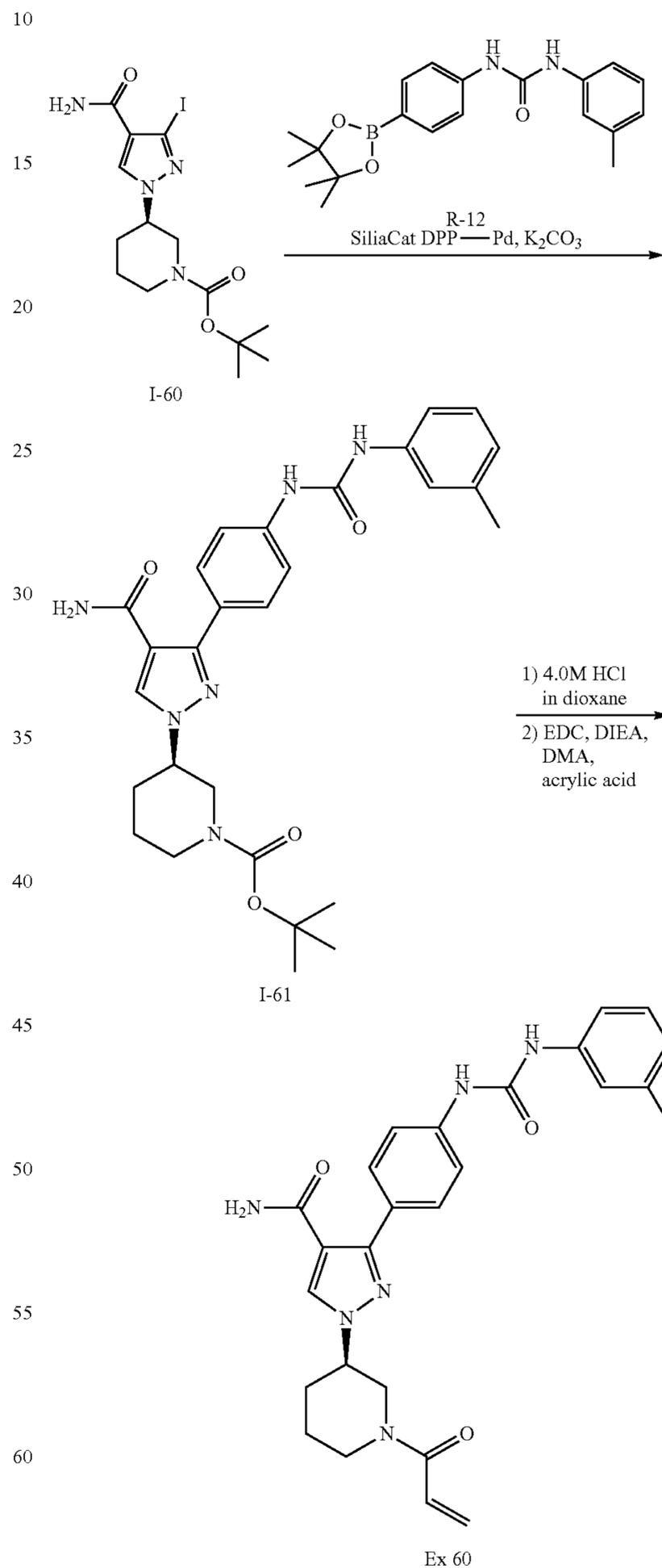
To a solution of I-60 (43 mg, 0.10 mmol) in DME (2 mL) is added R-12 (65 mg, 0.18 mmol), SiliaCat DPP-Pd (50 mg,
