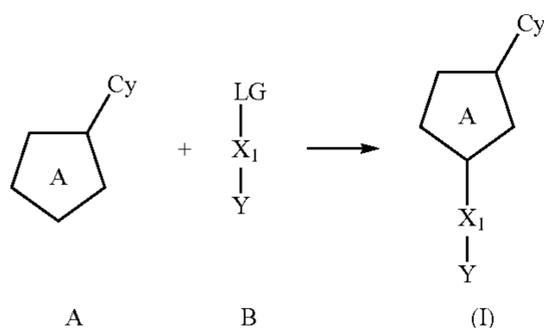
In scheme Ia, a heterocycle A is treated with a suitable base and reacted with an X<sub>1</sub>-Y group containing a leaving group (LG) B to afford the compound of general formula (I).
