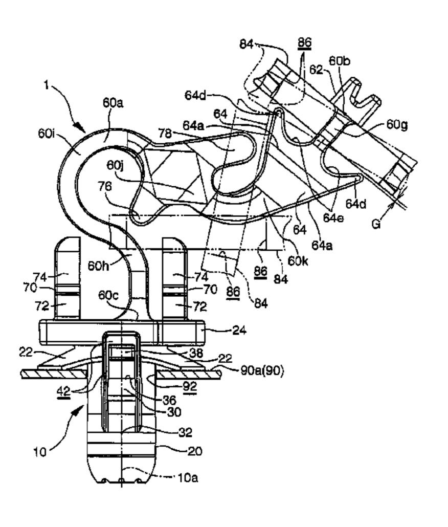
inserting aperture. When a bottom wall of the tether housing portion comes to a tether portion located between the guide plates and the anchor, the elastic branches and the protrusions prevent rotation of the tether. The second and third guide plates also prevent rotation of the tether.
