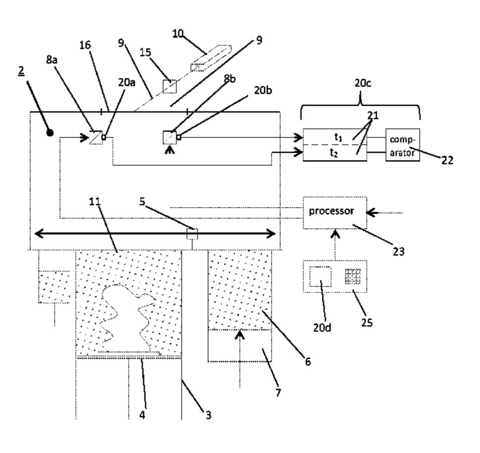
paring the irradiation times and/or irradiation areas of the scanners with each other; re-determining the surface sections of a powder layer to be irradiated by each scanner so the irradiation times for each scanner are approximated to each other and/or the irradiation areas of each scanner are aligned.
