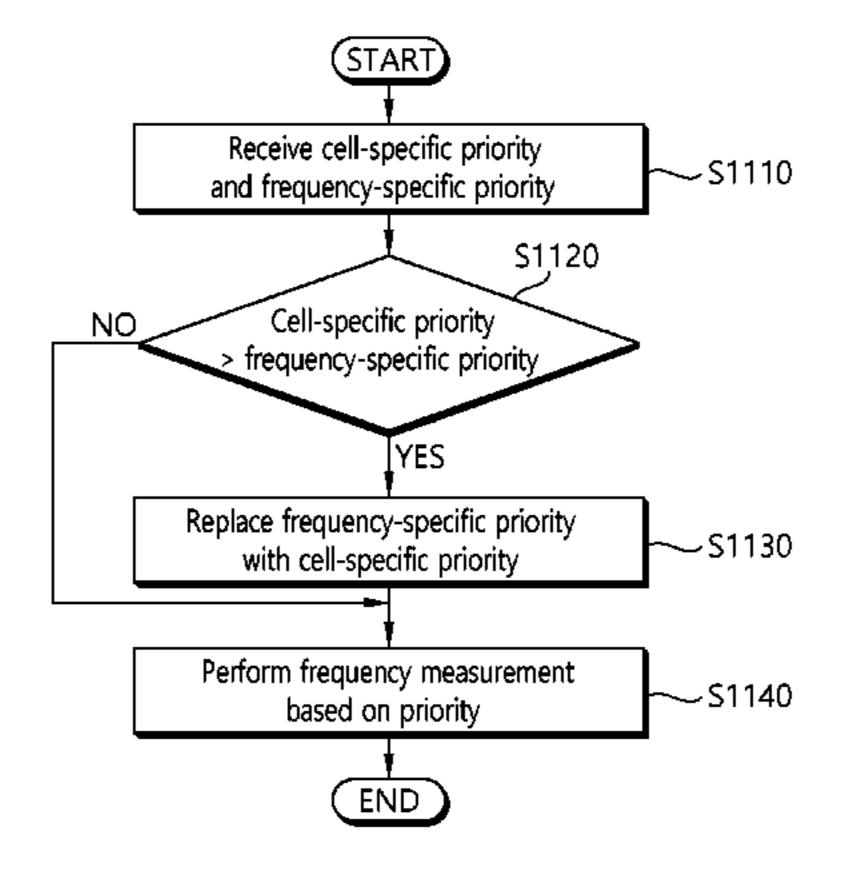
and a frequency specific priority of the frequency to which the first cell belongs; determine whether to apply the cell specific priority of the first cell to the frequency to which the first cell belongs; and perform frequency measurement on the basis of the determined priority. The first cell is a cell for which a cell specific priority is set, and the cell specific priority may be set to be the same for each frequency.
