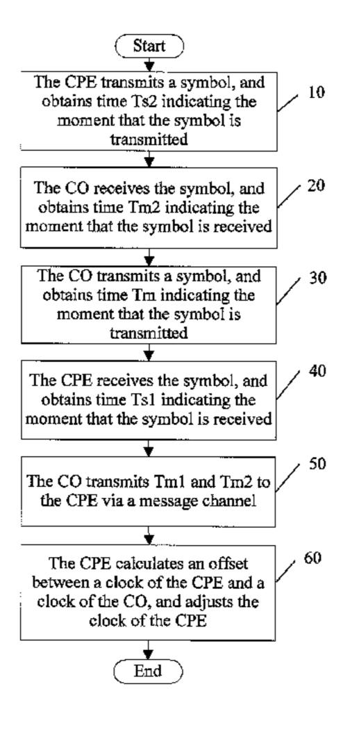
CPE calculates an offset between a clock of the CPE and a clock of the CO according to Ts1, Ts2, Tm1 and Tm2; and the CPE adjusts the clock of the CPE according to the offset to achieve synchronization.
