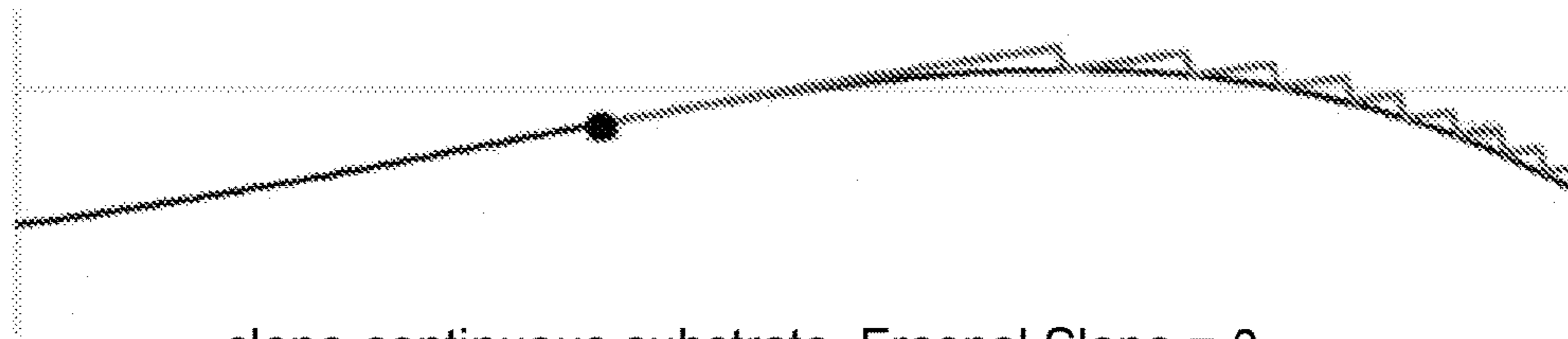
slope-continuous substrate, Fresnel Slope = 0
