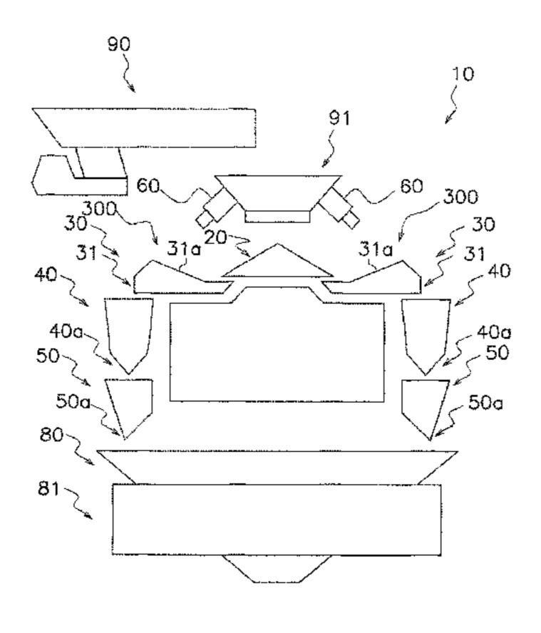
radial feeders (30), and in an obliquely downward direction from an upstream side to a downstream side in the conveyance direction of the articles.
