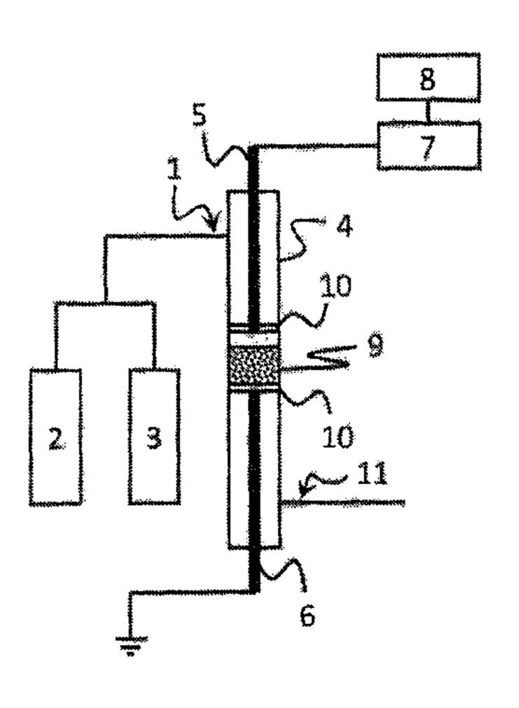
ammonia, and applying a voltage to the electrodes of the reactor for synthesizing ammonia, wherein electrical discharge does not occur by the voltage.
