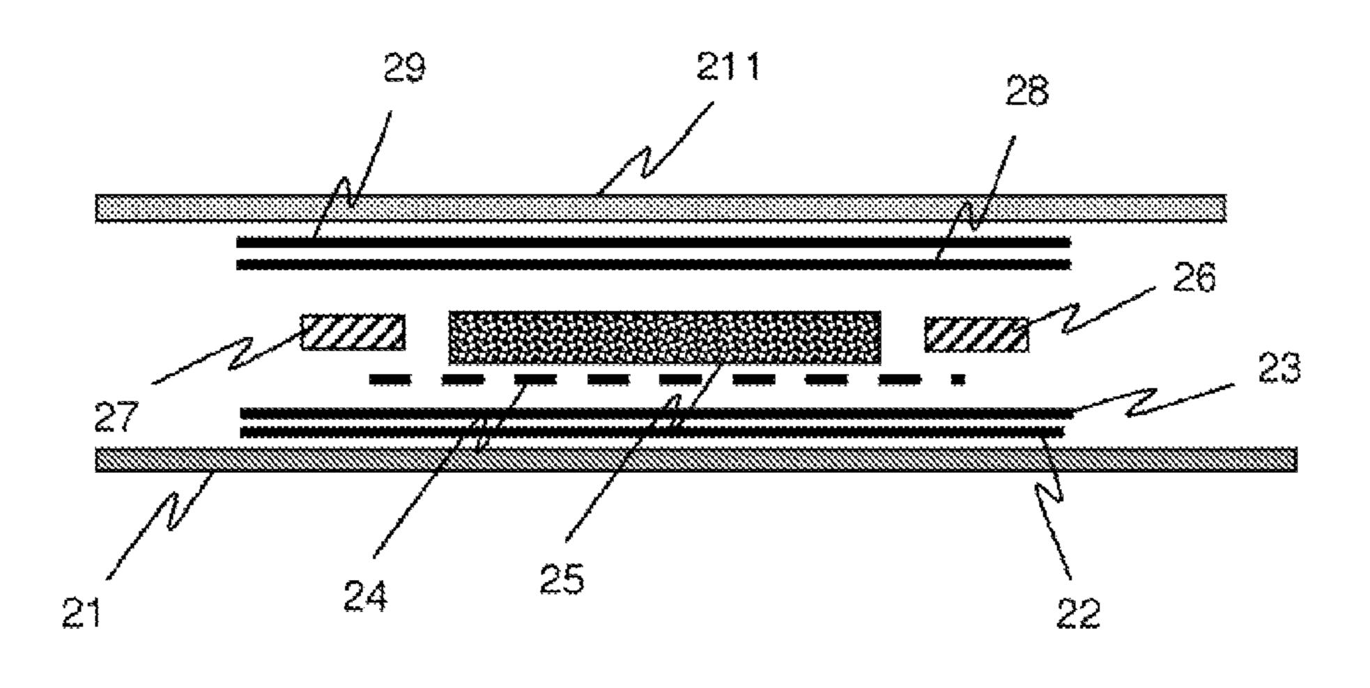
between the surfaces of the elastomer and the composite that are welded to each other, and passing an electric current through same, resulting in the surface melting of the two materials.
