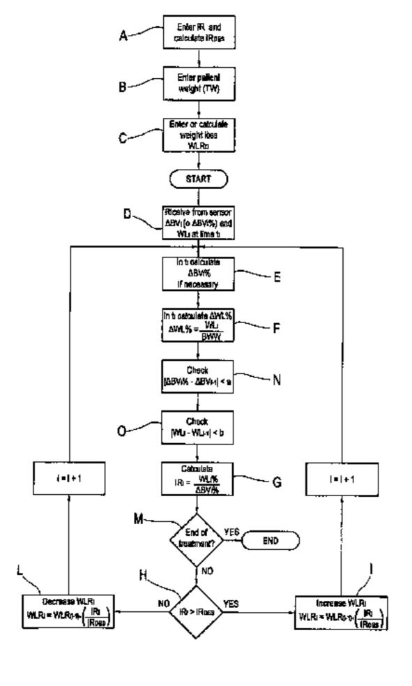
and the relative variation of weight loss (AWL/TW) of the individual with a desired value, and controls the weight loss of the individual on the basis of the comparison. The apparatus enables automatically controlling a dialysis, preventing some complications due to hypotension.
