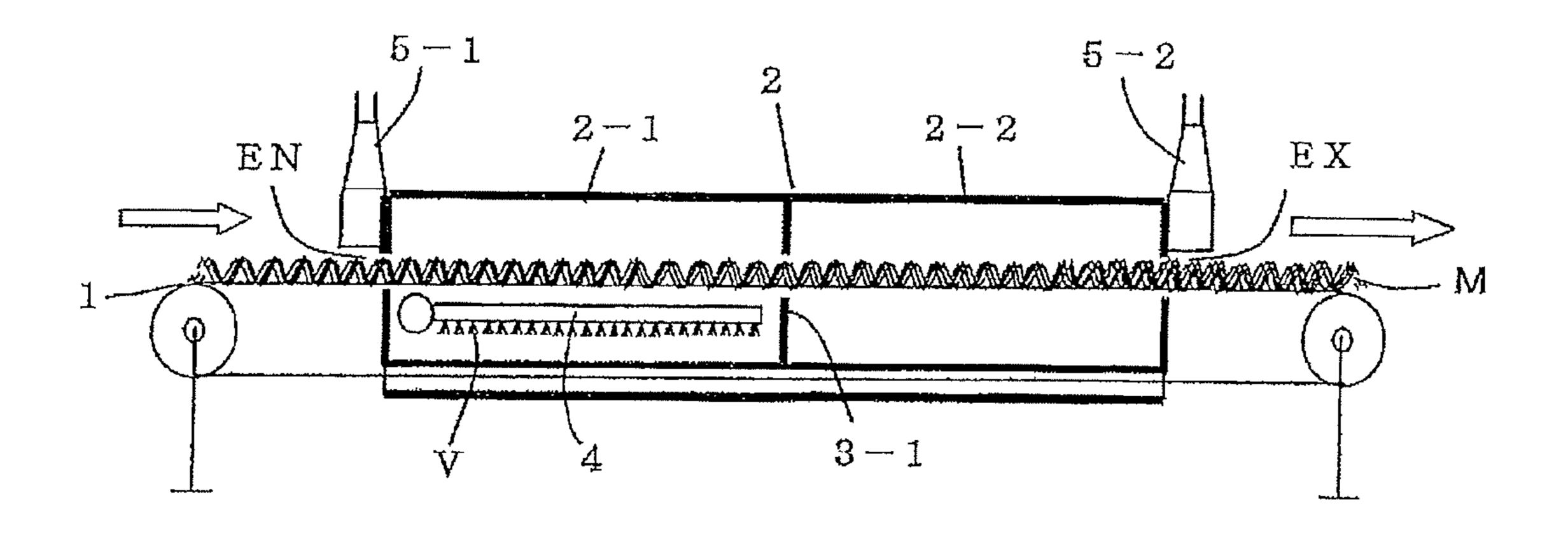
supplying the steam, and then transporting the bunch of noodle strings to an exit portion, and a noodle strings steaming device performs the above method.
