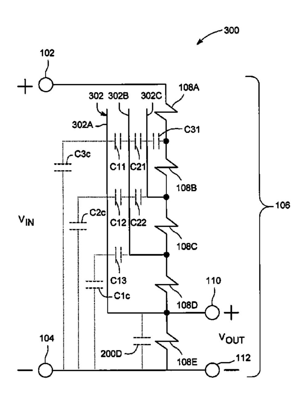
shield. A first internal resistor is disposed inside the external shield and outside of the internal shield(s). One or more remaining resistors are inside the internal shield(s). The shields divide parasitic capacitances to enable the measurement of dynamically changing high voltage input signals.
