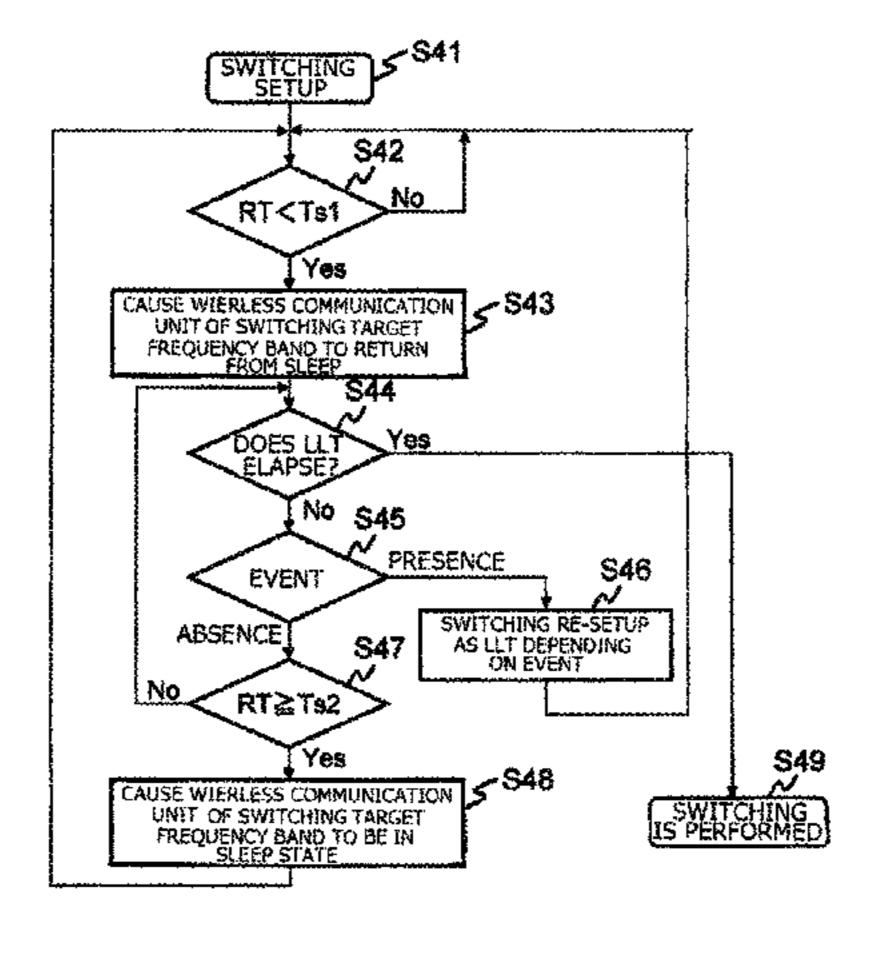
connection establishment, and the LLT is changed (LLT=T2 to T4) based on, for example, a state of transmission data or a change in a channel state.
