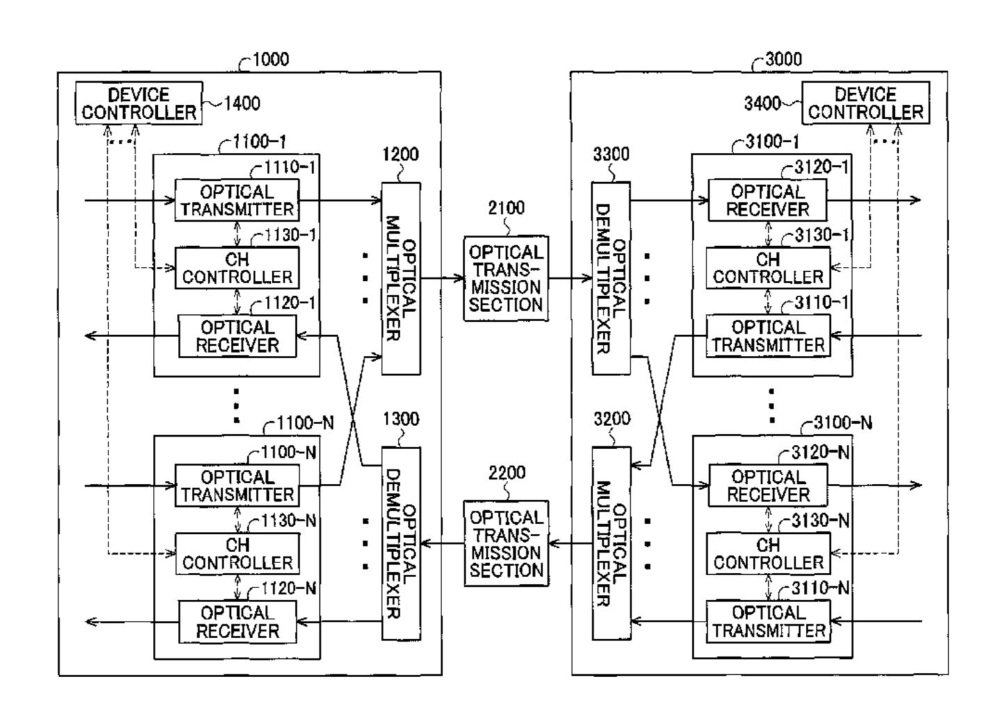
tion states of the multiple channels are correlated in the optical transmission section has a length such that an error rate is less than or equal to a threshold value, the error rate being determined from a temporal distribution of bit errors obtained from a result of error decision after demodulation in an optical receiver.
