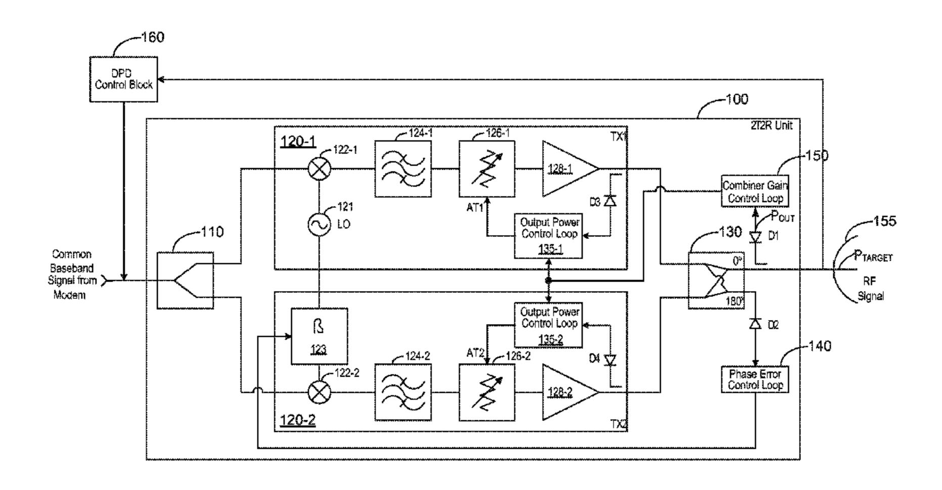
phase error control loop adjusts the phase shifter to minimize the 180-degree phase-shift radio-frequency output. A combiner gain control loop adjusts the output power level of the two transmitters in accordance with an actual power detector reading at the 0-degree phase-shift radio-frequency output.
