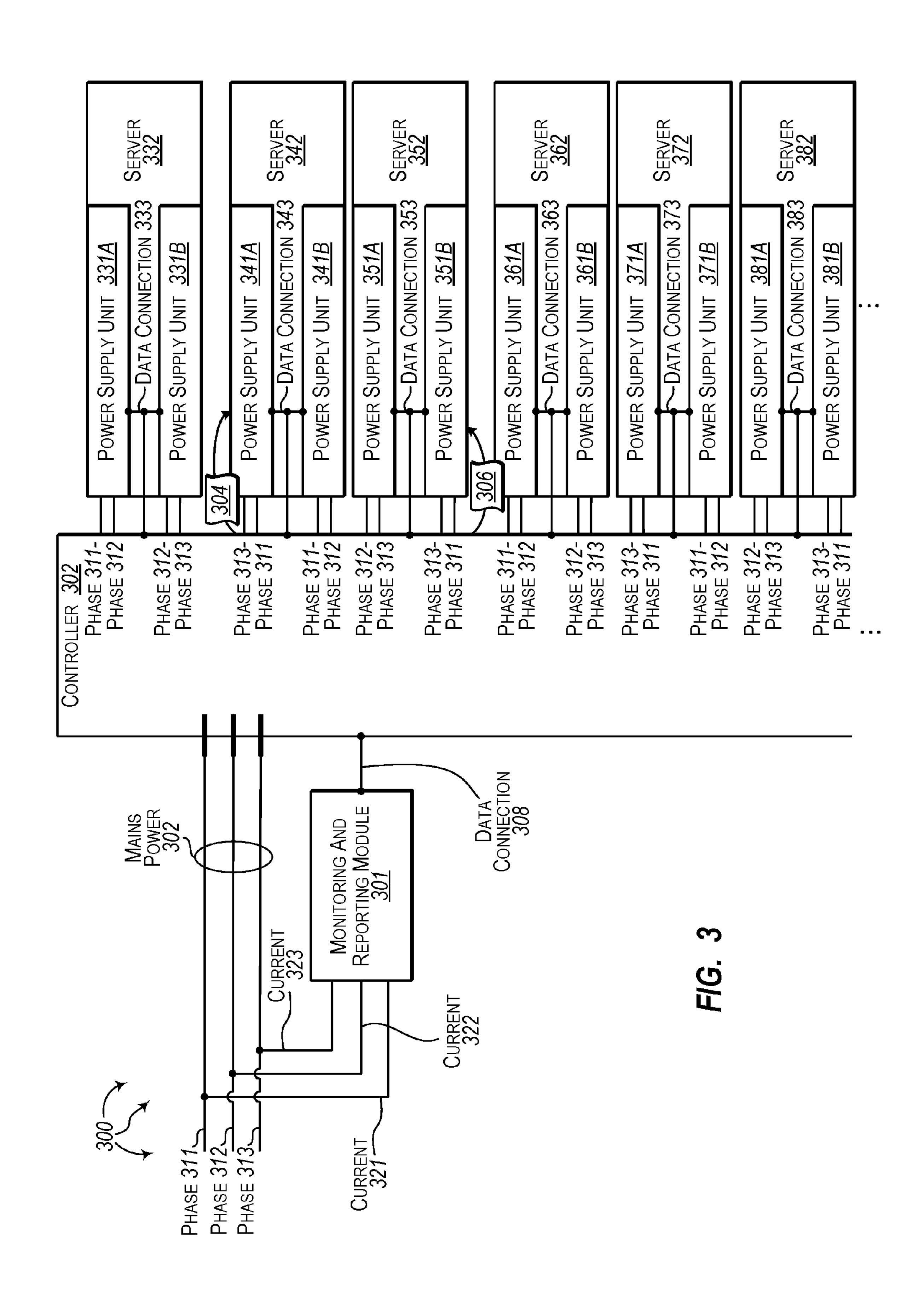
DETECTING THAT THE CURRENT FOR A FIRST PHASE IS IMBALANCED WITH AT LEAST ONE OF: THE CURRENT FOR A SECOND PHASE AND THE CURRENT FOR A THIRD PHASE
