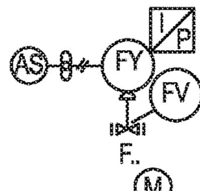
CONTROL VALVE DIAPHRAM ACTUATOR WITH ELECTRO-PNEUMATIC POSITIONER, ALSO AVAILABLE WITH CYLINDER ACTUATOR
