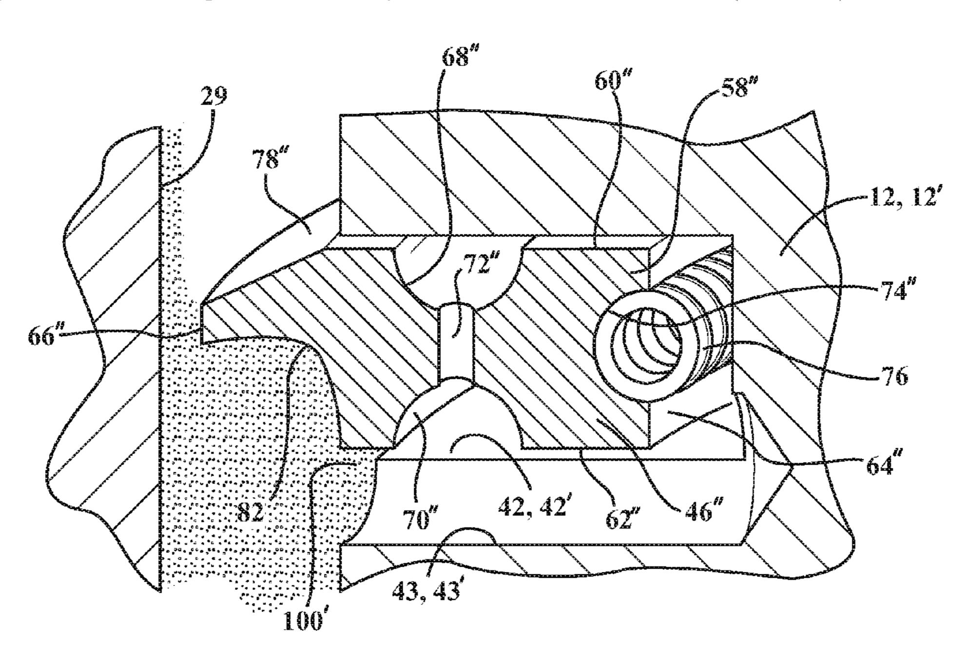
into fluid communication with one another. The annular grooves collect oil scraped from a cylinder wall and return oil to the crank sump and reduce the contact area between the oil control ring and the wall of the ring groove.
