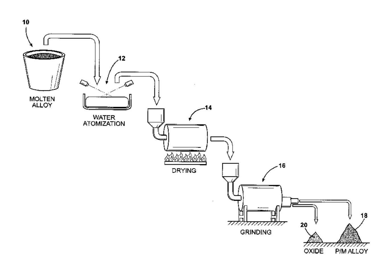
atomization. The powder metal composition includes metal carbides in an amount of at least 15 vol. %. The microhardness of the powder metal composition increases with increasing amounts of carbon and is typically about 800 to 1,500 Hv50.
