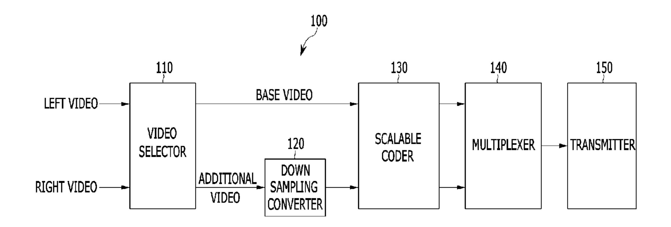
enhanced layer data by coding a correlation video between the base video and a video decodable from the base layer stream, and transmits the base layer data and the enhanced layer data.
