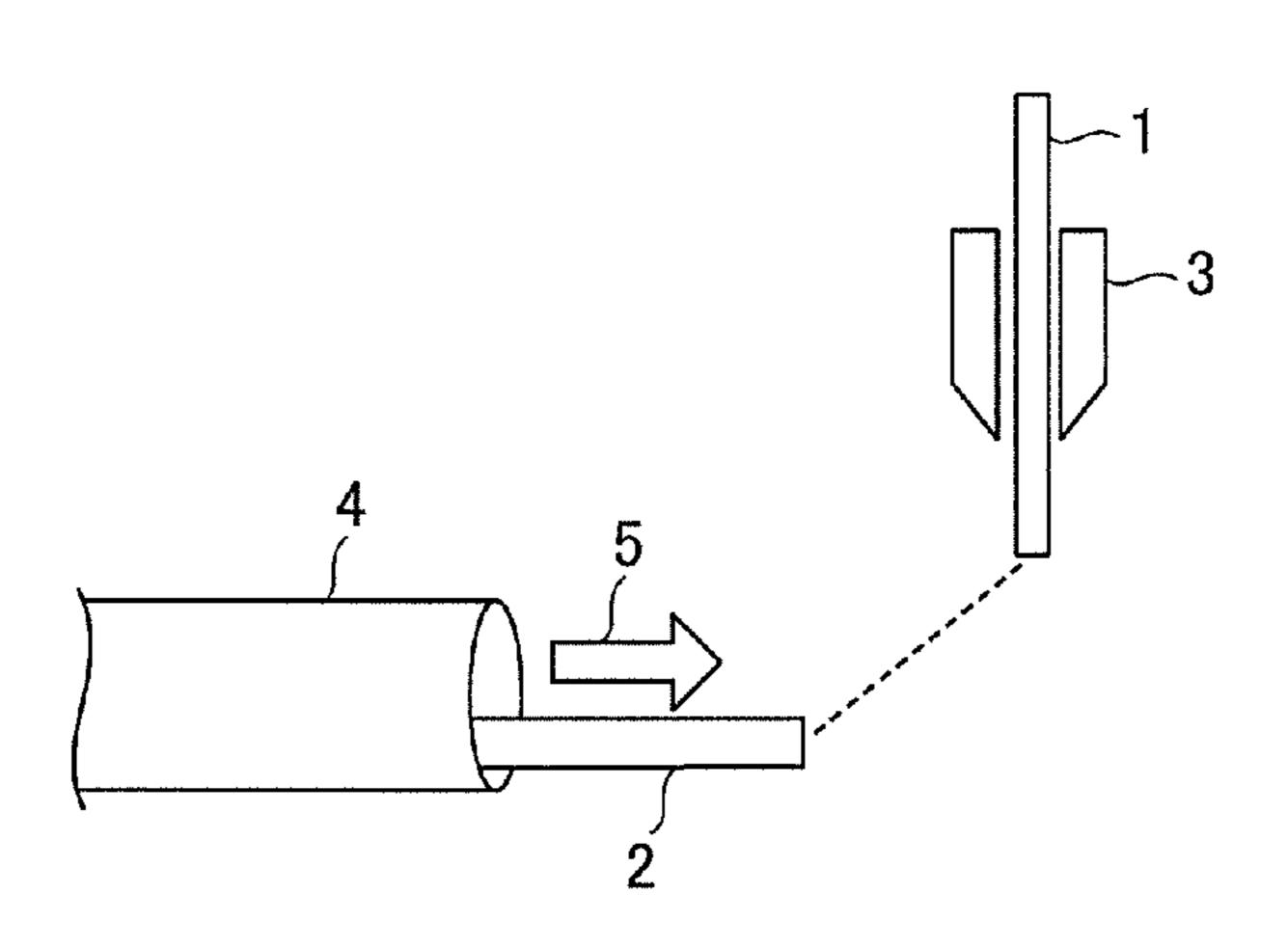
pressure, the method being capable of improving Pd coverage on a ball surface in forming a ball at a tip of the Pd-coated Cu bonding wire.
