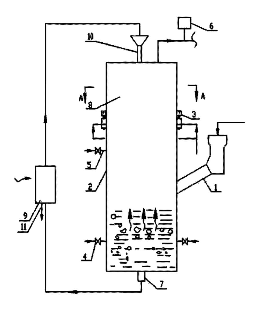
zone of the furnace body, and the lower nozzle for spraying CO<sub>2</sub>/vapor is disposed in a bed zone of the furnace body. The monitoring unit is disposed close to the syngas outlet. The one or two layers of microwave plasma generators are disposed above the upper nozzle in the clearance zone of the gasifier.
