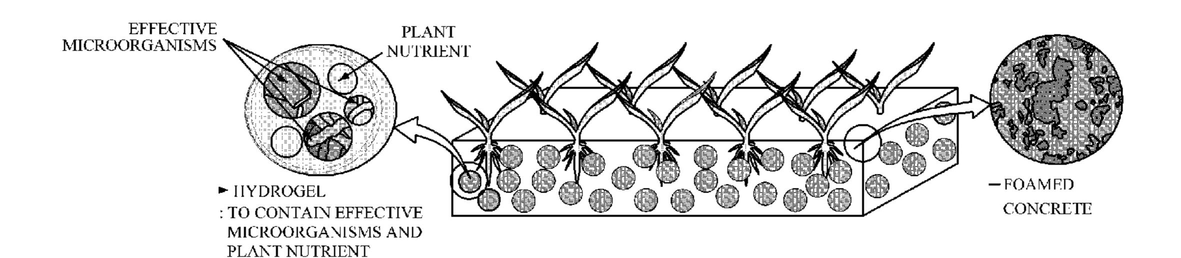
concrete. When the foamed concrete is used, a designated compressive strength can be ensured and a number of pore spaces are formed, which allow the air to be sucked and expelled therethrough and store moisture therein. Also, hydrogel that is incorporated into the foamed concrete may supply nutrients required for plant growth, improve pest resistance, and store and supply a large amount of water.
