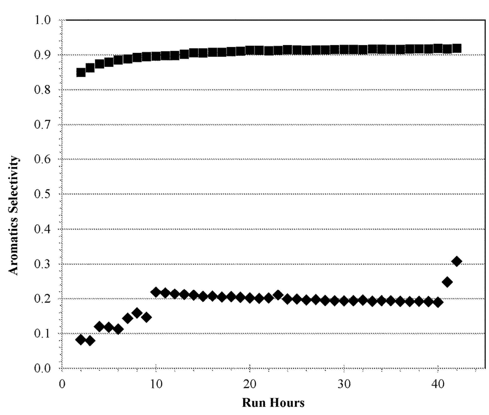
■ Fresh catalyst of Example 1 ◆ Sulfur-contaminated catalyst of Example 2
