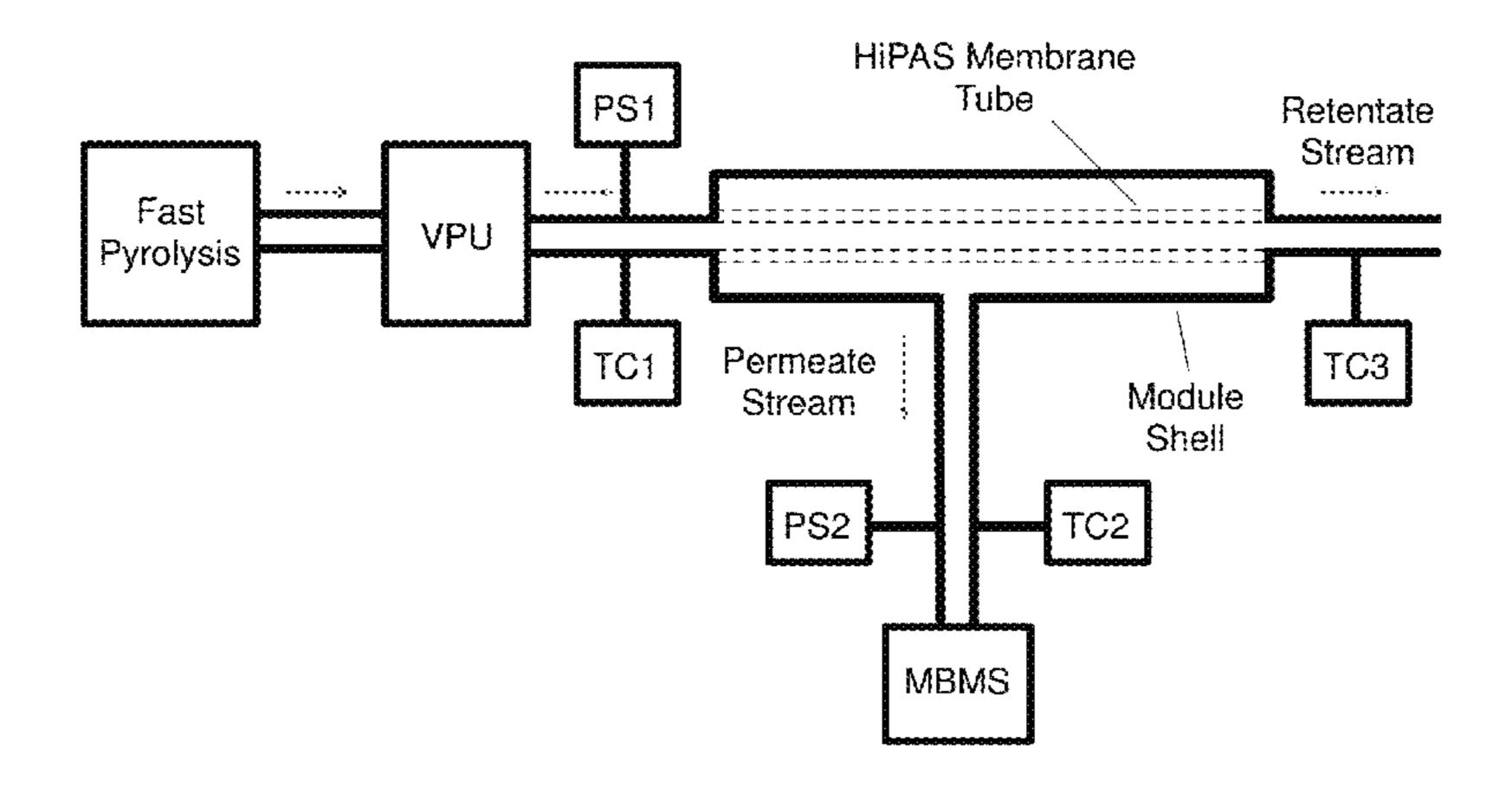
particularly directed to embodiments where the heated vapors emanate from a pyrolysis process. An apparatus for achieving the above-described method is also described.
