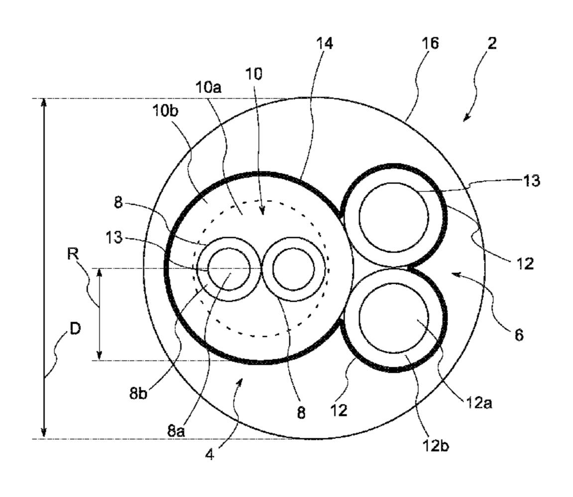
sleeve, which is in turn surrounded by a common sheath of the electric lead. The lead is characterized in that the partial lead sheath has an inner sheath section and an outer sheath section, and the outer sheath section is harder than the inner sheath section.
