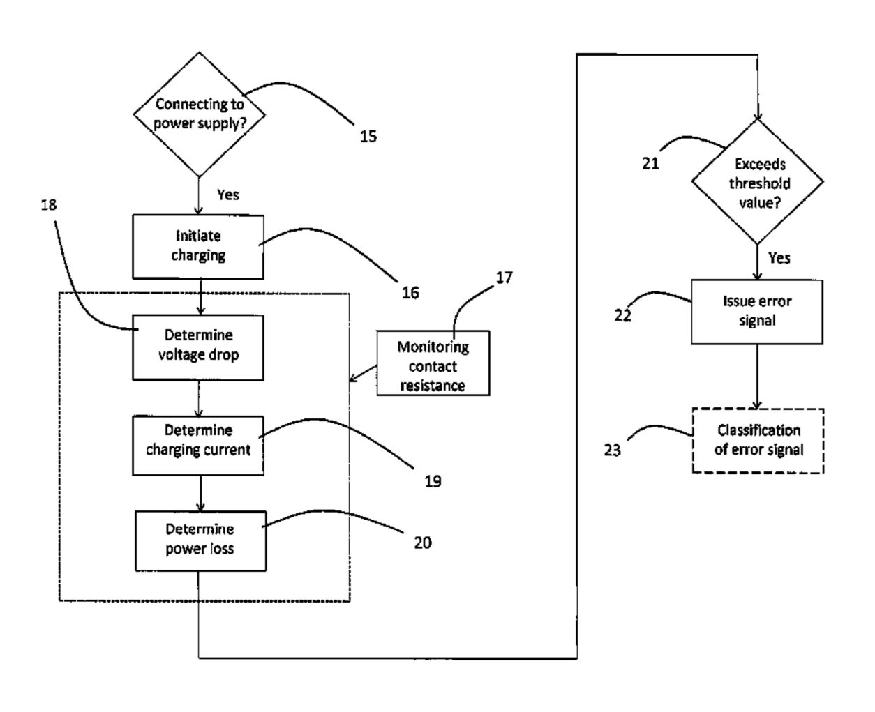
the method includes measuring and calculating the power loss over the connector elements during the charging, and generating an error signal if the power loss is higher than a predetermined threshold value, the error signal being dependent on the magnitude of the power loss. An arrangement for controlling charging of an electric energy storage system in a vehicle is also provided.
