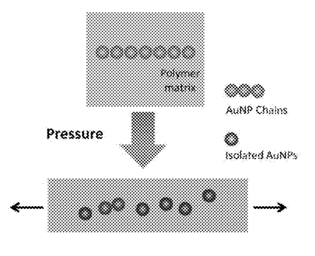
used to capture and record the pressure distribution and magnitude between two contacting or impacting surfaces by outputting color information.
