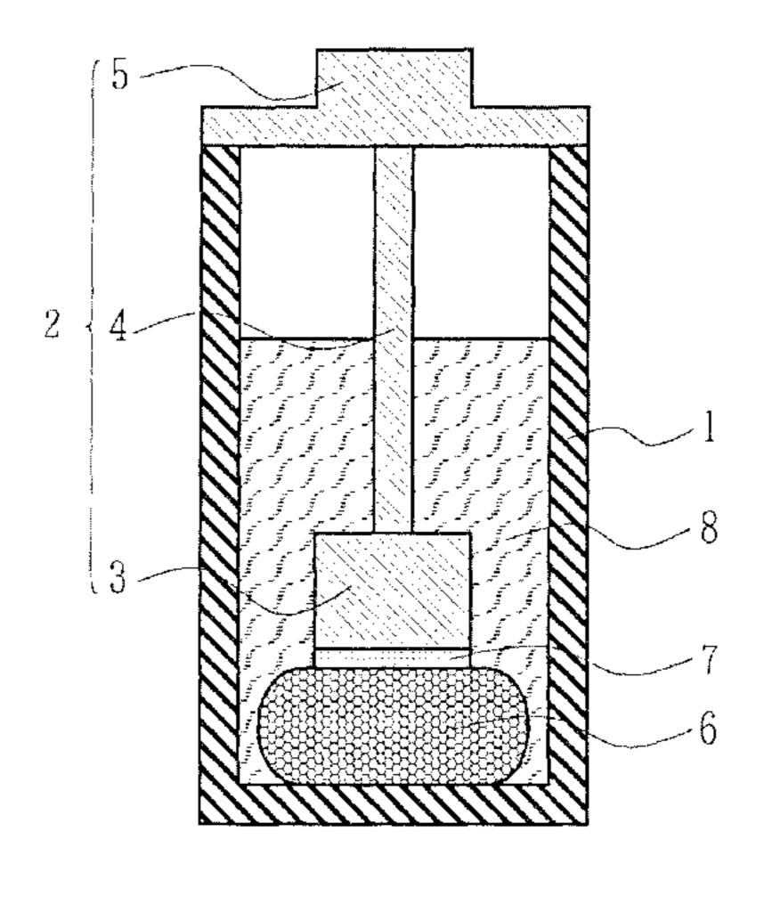
wherein the fixing buffer member exerts a buffering effect in the liquid nitrogen.
