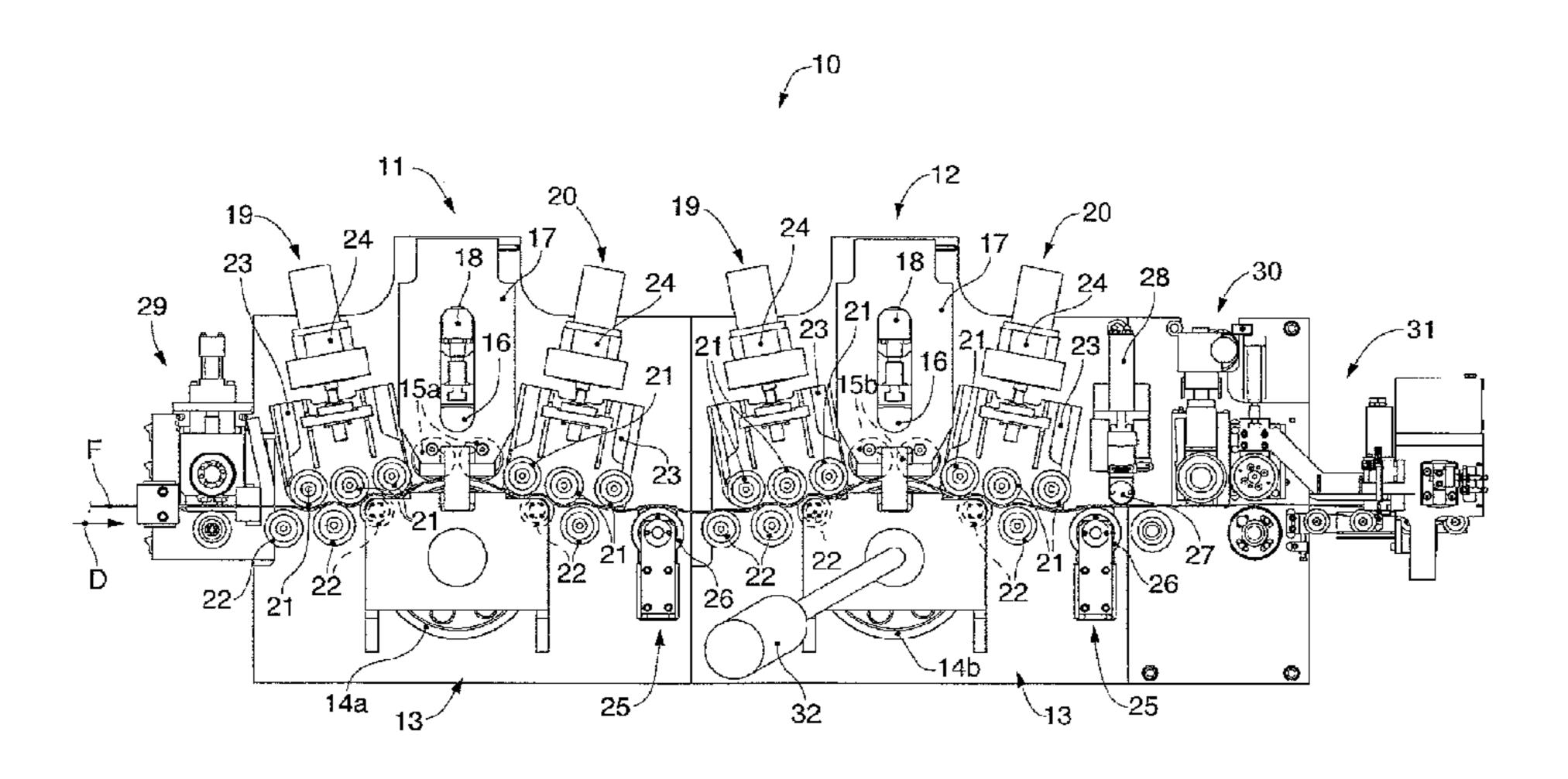
main roll, on part of the periphery of which second idle contrast rolls are disposed, with a diameter smaller than the second main roll.
