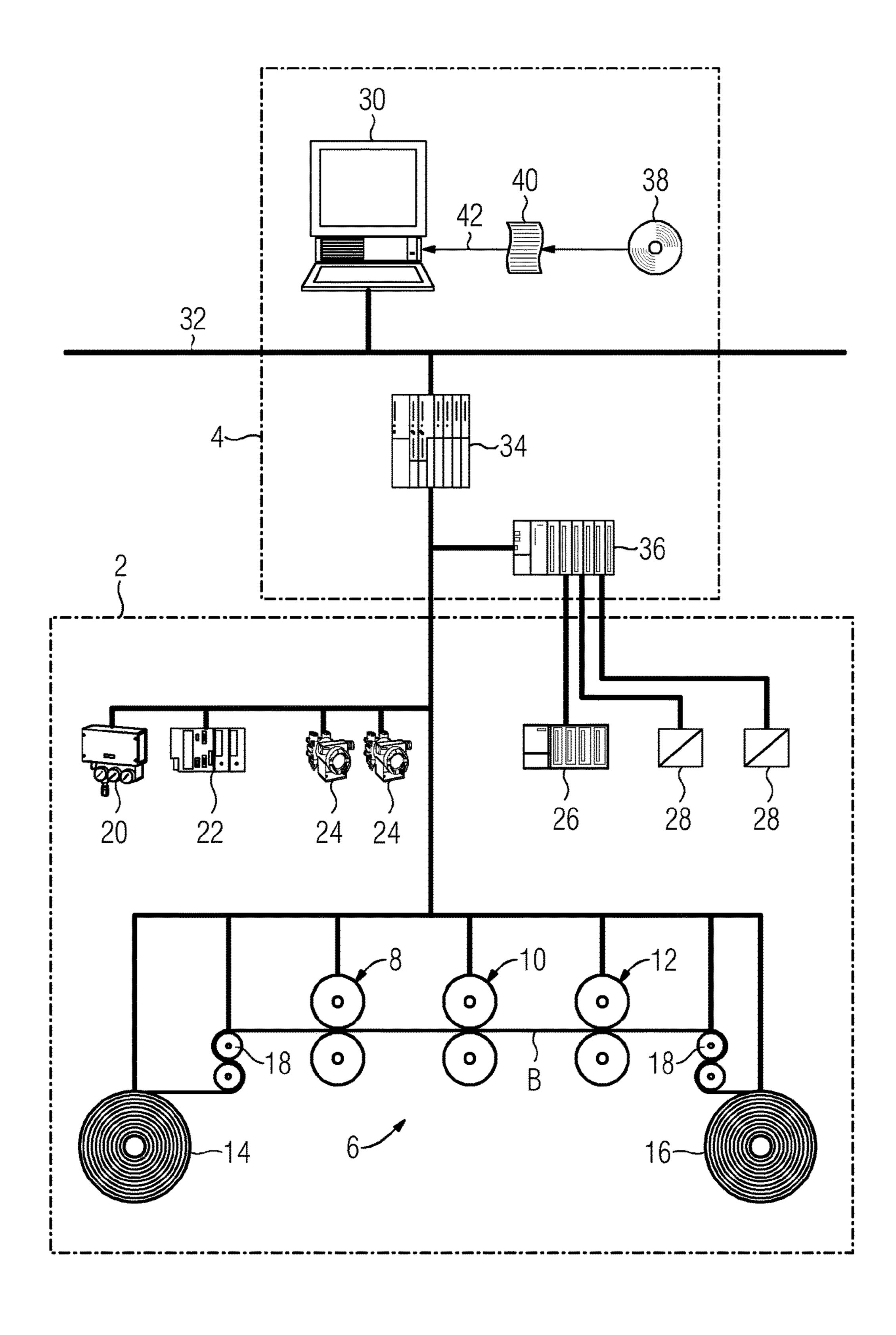
METHOD FOR REDUCING THE ENERGY CONSUMPTION OF A ROLLING MILL INSTALLATION, CONTROL AND/OR REGULATION DEVICE FOR A ROLLING MILL INSTALLATION, MACHINE-READABLE PROGRAM CODE, STORAGE MEDIUM AND A ROLLING MILL INSTALLATION
