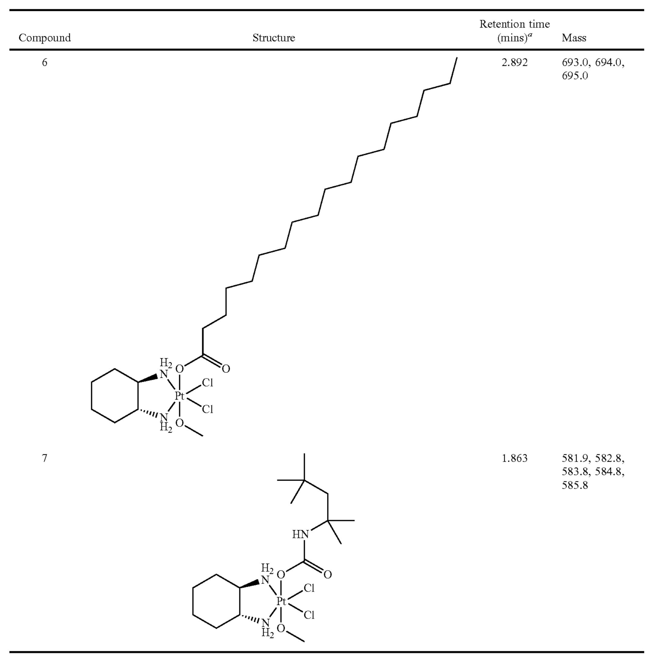
"HPLC/MS conditions: Mobile Phase: A: water (0.01% TFA) B: ACN (0.01% TFA); Gradient: 5%-95% B in 1.4 min; Flow Rate: 2.3 mL/min, 3.2 minute run; Column: SunFire C18, 4.6 × 50 mm, 3.5 μm; Oven Temperature: 50° C.
