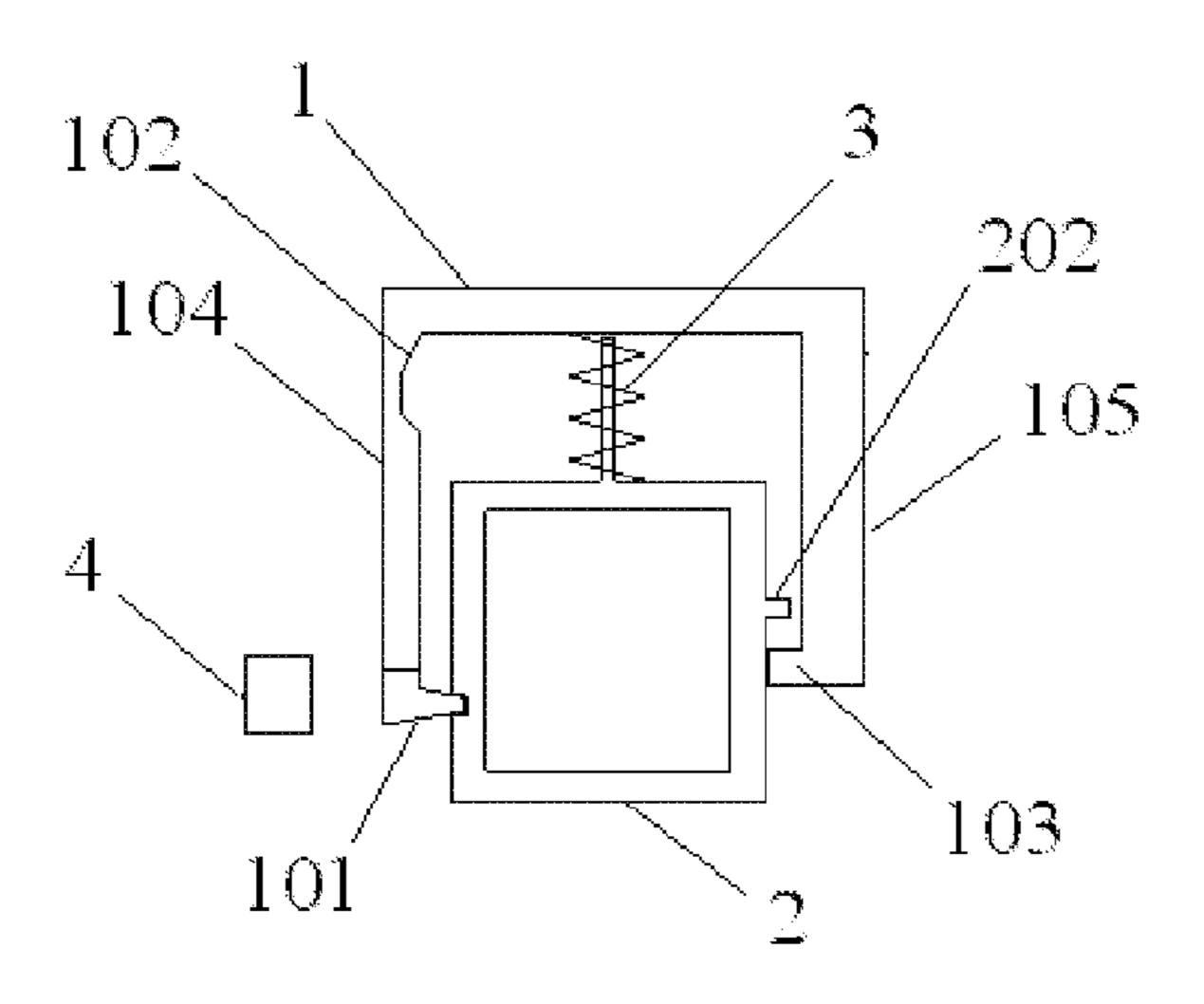
to eject the stopper body, the system further includes a magnetic module, and the magnetic module is an electromagnetic module, and attracts the limiting lug boss to be separated from the limiting groove when being energized. The system for ejecting the stopper of the mobile terminal implements automatic ejecting of the stopper of the mobile terminal.
