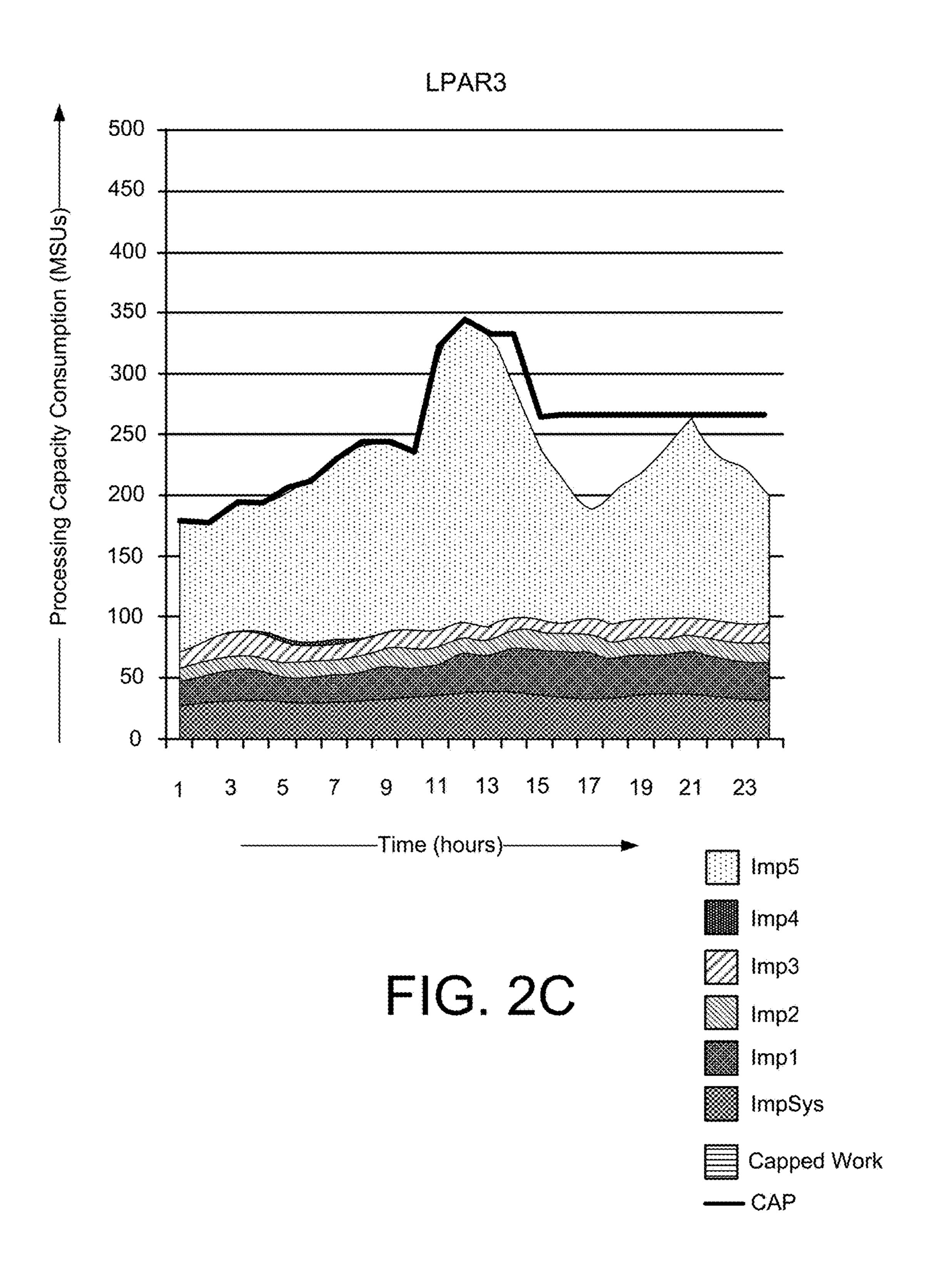
Querying a Workload Manager (WLM) component of the LPAR O/S to determine recent consumption of MSUs by importance level of work for each entity (e.g., LPAR or capacity group) in the managed group of system usage entities 310
