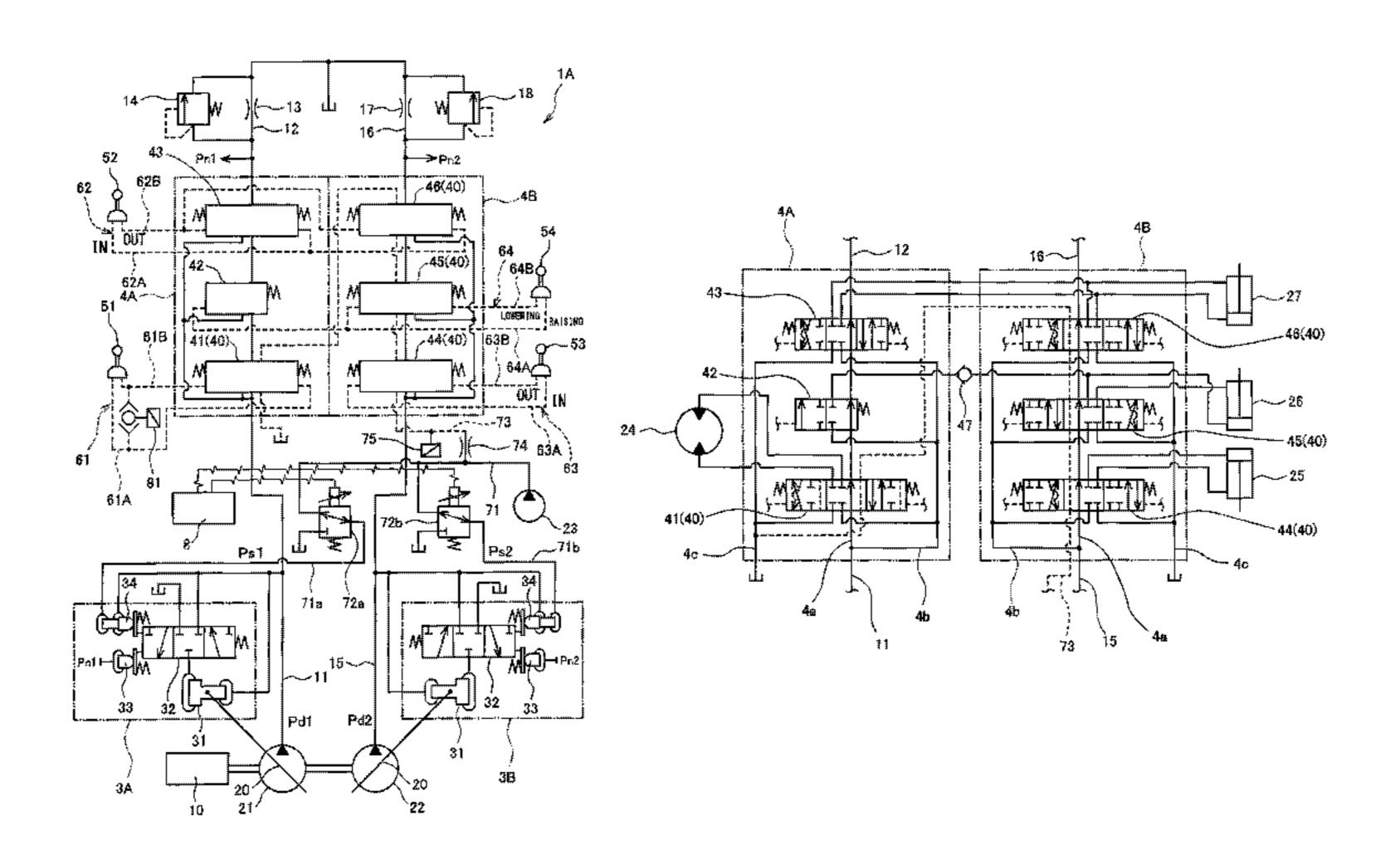
shift pressure is set by a first proportional valve, and the second power shift pressure is set by a second proportional valve.
